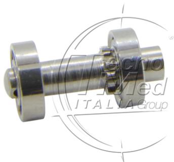
Compatible Sirona low speed handpiece rotor for T1 Line C200/L, T2 Line A200/L, T2 Line A170/L and T3 Line E200/L, with 13 Z gear Ø 9.7mm, with Myonic torlon ceramic bearings.
